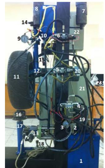
Fig. 4. General setup of the hydro-pneumatic suspension system
