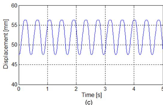
Fig. 9. Experimental results of the controlled System at 60 kg (a) proportional valve current, (b) cylinder pressure, and (c) suspension displacement
