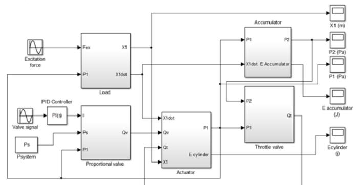
Fig. 2. The Simulink model of the quarter car model's suspension
