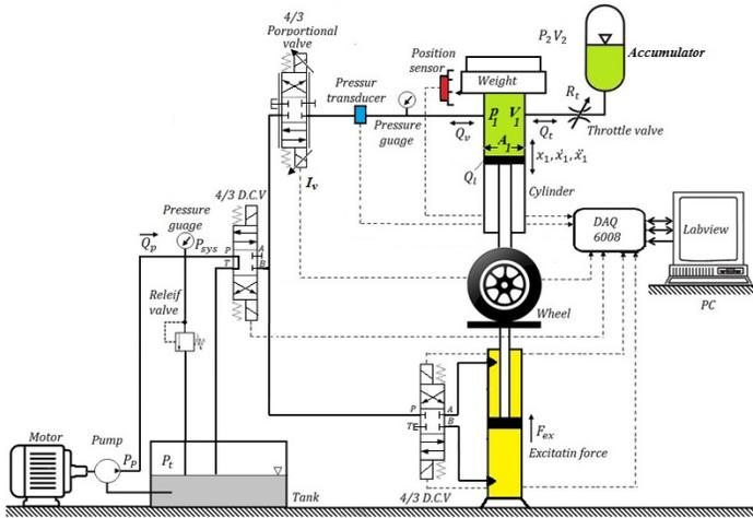
Fig. 1. General setup of the hydro-pneumatic suspension system
