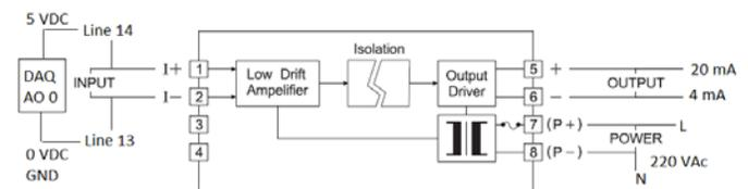
Fig. 5. Signal isolated transmitter and wiring connection
