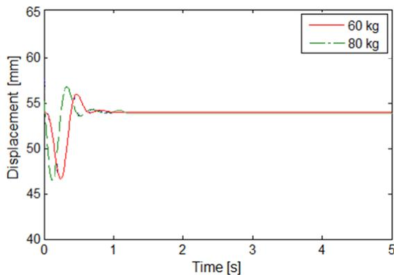
Fig. 8. Disturbance rejection of car body when subjected to additional weight
